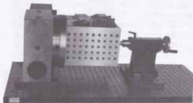
Stevens 4-Sided Column with Stevens Modular Vise is shown above mounted on Haas headstock and tailstock.
