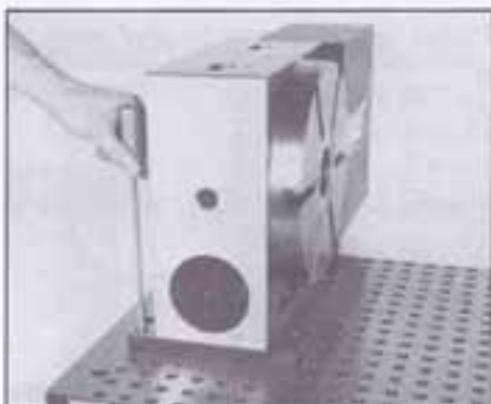
Standard Stevens Tooling Plates can generally be used as headstock adapters. See pages 29 and 30 for stock Tooling Plate sizes.
