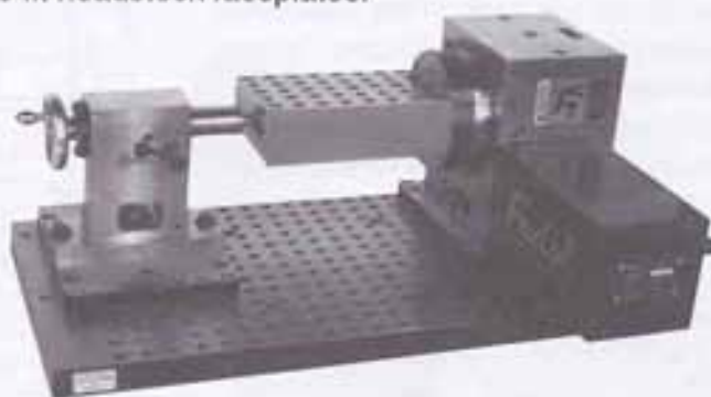
The 2-Sided Plate (shown above) is advantageous for larger workpieces requiring greater swing clearance.
