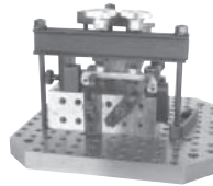
Qualified edges of Small Utility Block are used here to establish secondary and tertiary locations.
